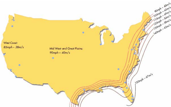
Fig. 1: Maximum 50-year Wind Speeds in the United States Based on International Building Code Data.
