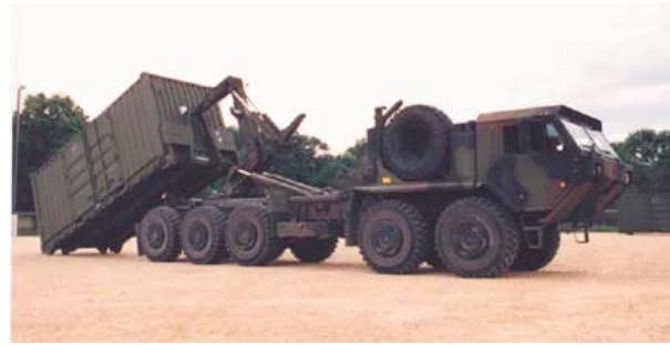
Figure F: U.S. Army Truck Equipped with a Palletized Load System to handle a 20-ft. ISO Container.
