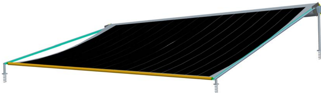
Figure E: A Single Retractable Roll Assembly Showing Saddle Shape
